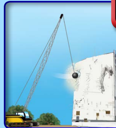
A wrecking ball on a short chain (above) cannot be lifted as high and hits the wall with less energy than a wrecking ball on a longer chain (right).
